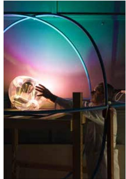
EMC Test - Triple Loop Antenna
