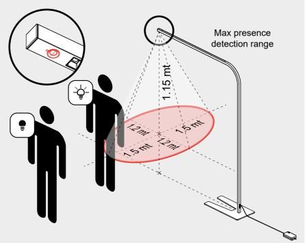
If the user leaves the lamp on and walks away, after 10 minutes, light emission lowers to 30%; then after a further 3 minutes, the lamp switches off.
