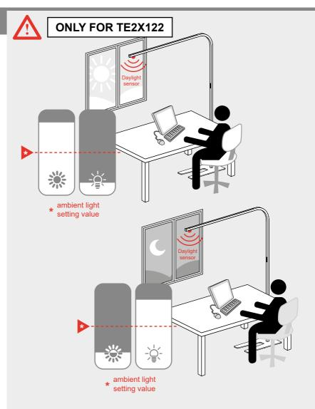
The luminaire is equipped with a daylight sensor and PIR sensor. The luminaire comes with a pre-set **ambient light setting** in memory.
