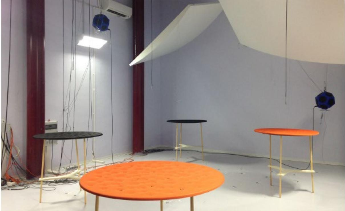
Figure 2: Arrangement of the 4 Silent Field lamps in reverberant chamber.
