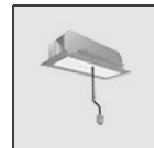
240W Recessed power supply kit (cable length 2,2 m) - 230VAC-48VDC - IP20 - 396x195x112H - White - Undimmable AQ17401
