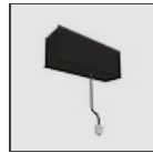
150W Ceiling power supply kit (cable length 2,2 m) - 230VAC-48VDC - IP20 - 321x91x111H - Black - DALI AQ17504
