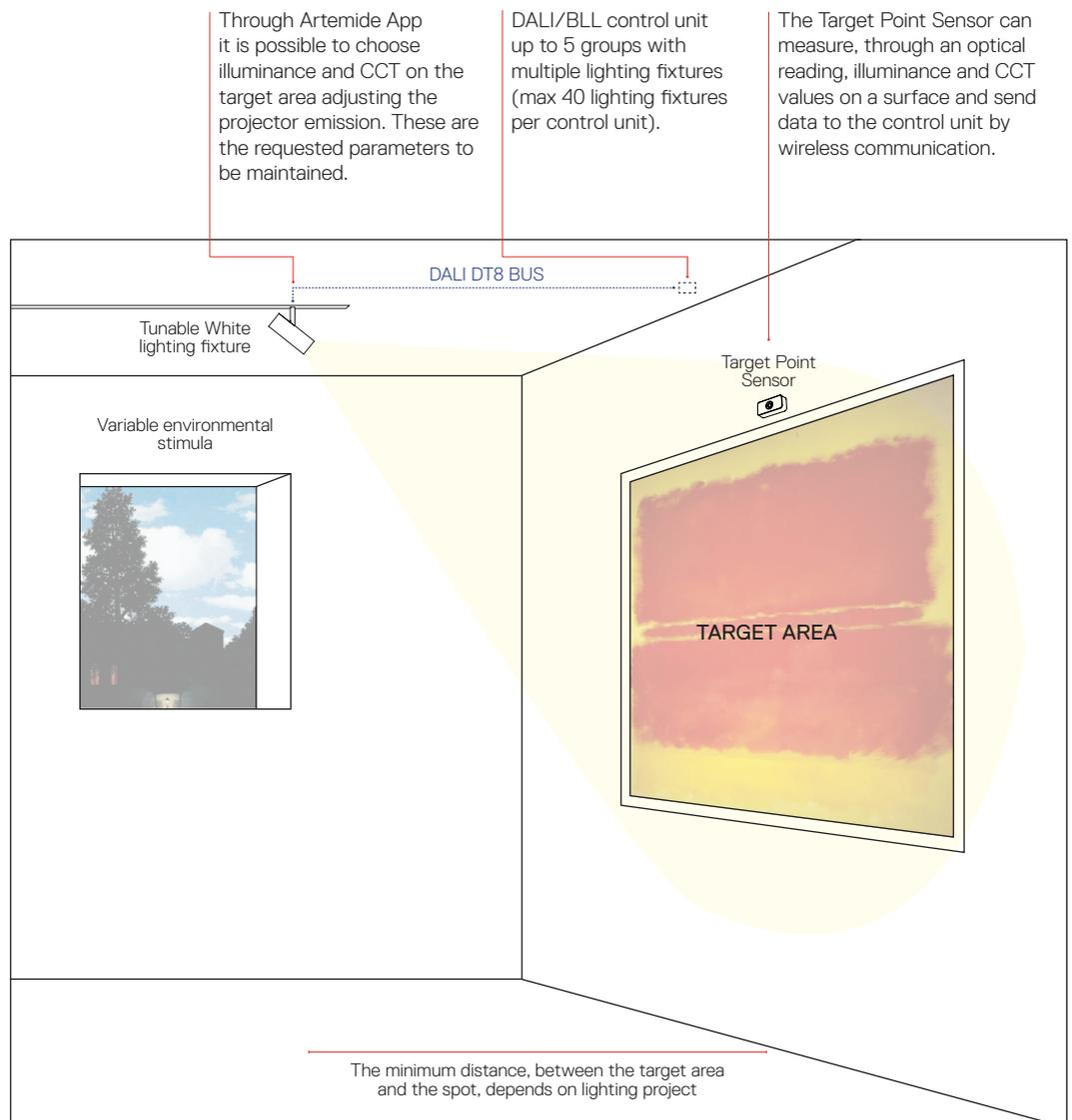
The Target Point system allows to ensure the constant illuminance and color temperature of a specific target area whatever the environment conditions.
