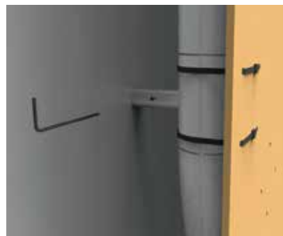
5. Detail of the wall pins fixing.
