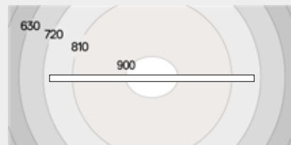
A.39 Sharp microrefractive emission - black louvres 1184 mm - direct only Installation h 2400 mm - Desk h 750 mm Isolines (lx) on a desk 1600x800 mm
