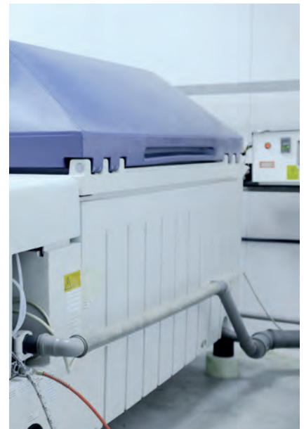
Corrosion Test - Salt-acetic fog chamber
