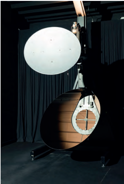
Photometric Measurements - Goniophotometer with rotating mirror
