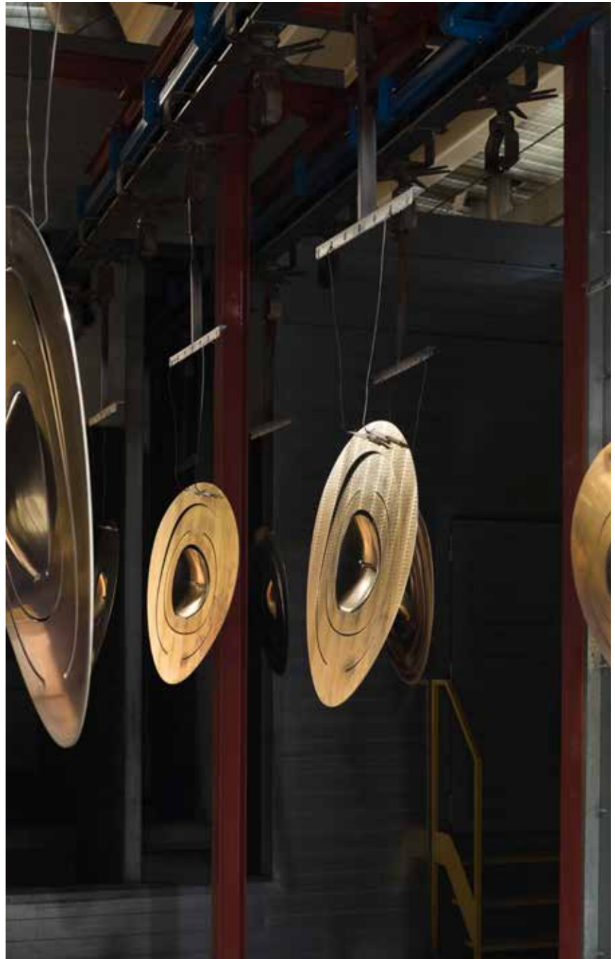
Coating Machinery - Artemide Factory Pregnana Milanese
