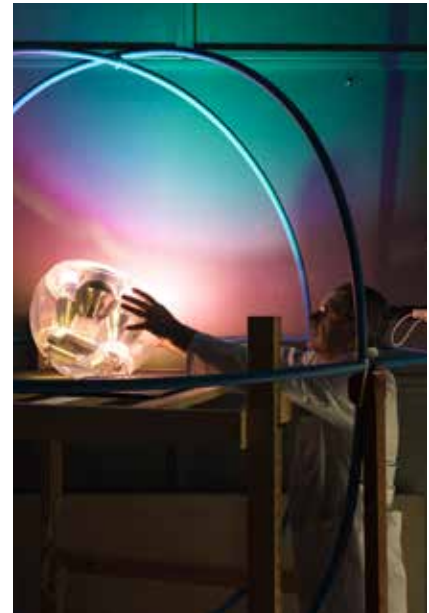
EMC Test - Triple Loop Antenna
