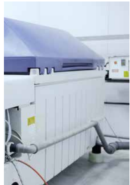
Corrosion Test - Salt-acetic fog chamber
