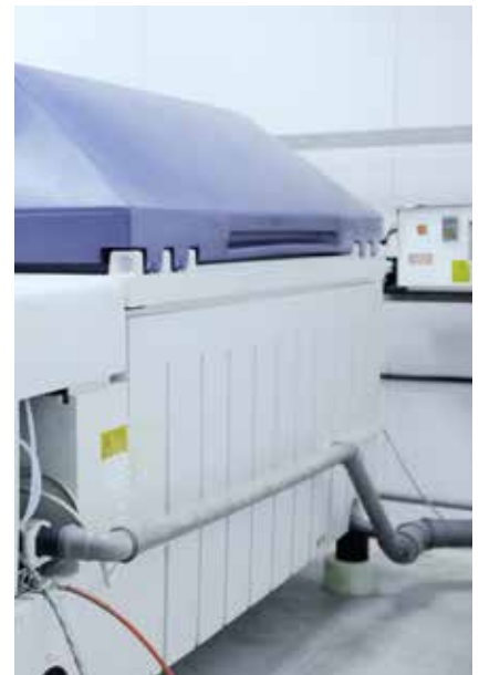
Corrosion Test - Salt-acetic fog chamber
