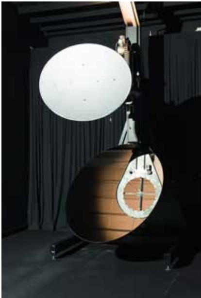
Photometric Measurements - Goniophotometer with rotating mirror
