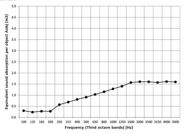
Figure 3: Frequency trend of absorbent units per object A
