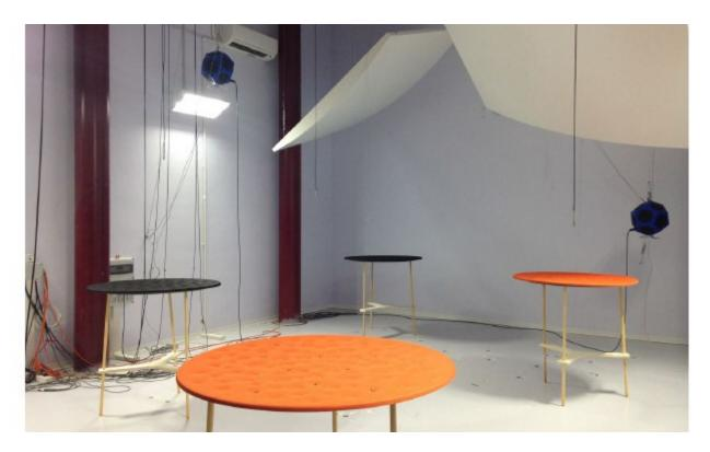
Figure 2: Arrangement of the 4 Silent Field lamps in reverberant chamber.
